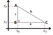
Suppose that  $A(x_A, y_A)$  and  $C(x_C, y_C)$  are two points in the plane. Consider the right-angled triangle ABC where  $B(x_A, y_C)$ . By the Pythagorean Theorem:  $AC^2 = AB^2 + BC^2$   $AC^2 = (y_C - y_A)^2 + (x_C - x_A)^2$ Hence:  $AC = \sqrt{(y_C - y_A)^2 + (x_C - x_A)^2}$ .
